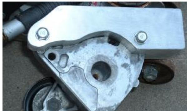
**Caution: DO NOT OVER TIGHTEN. ALWAYS TIGHTEN the bolt on the back first prior to installing. Nice hand tight is good. Using the power steering oem torque setting is recommended**
